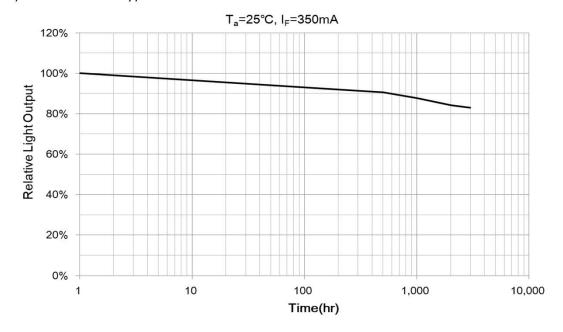
This life data was measured with the AIN submount on Al-substrate and fan.
