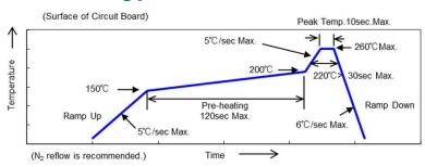
This soldering profile is according to JEDEC-J-STD-020D.
