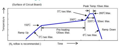
This soldering profile is according to JEDEC-J-STD-020D.
