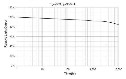
This life data was measured with the AIN submount on Al-substrate and fan.
