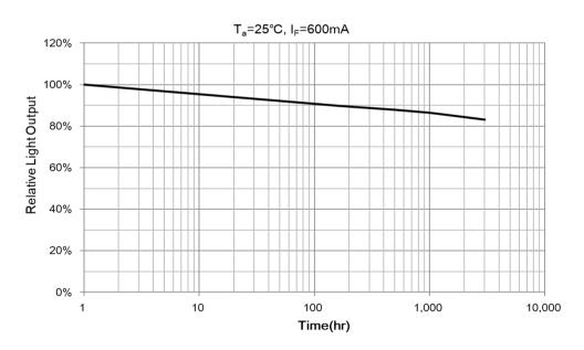
This life data was measured with the AIN submount on Al-substrate and fan.
